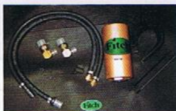
▲ Here are the contents of the Fitch Fuel Catalyst system we installed on Gonzolo Topete's '06 Mustang GT. The kit (PN F4424B; $224.45) includes everything needed for a quick and easy installation, save for Teflon sealant for the quick-connect fittings and a fuel-line disconnect tool.
